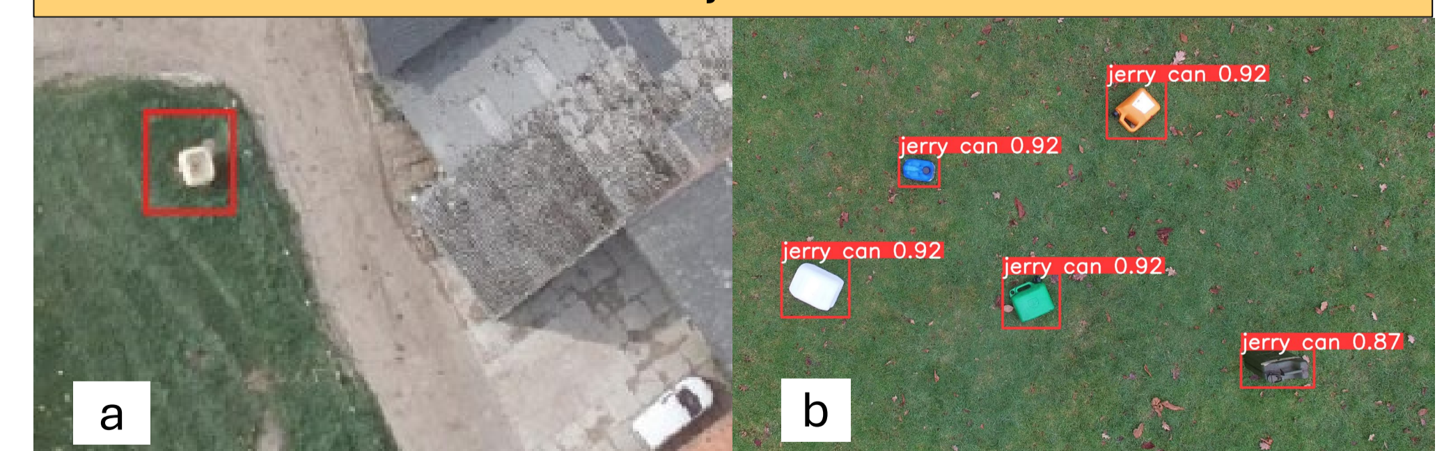
Figure 4: Detected objects using YOLOv8 algorithm trained on custom dataset : (a) IBC, (b) Jerry cans
